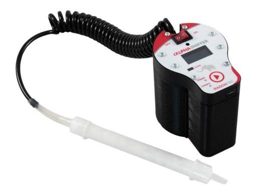
As radon decays inside the cell, the alpha particle emitted hits the wall of the cell, which is coated with scintillation powder, and emits a flash of light. The photomultiplier converts the light into an electronic pulse, which is then counted.
